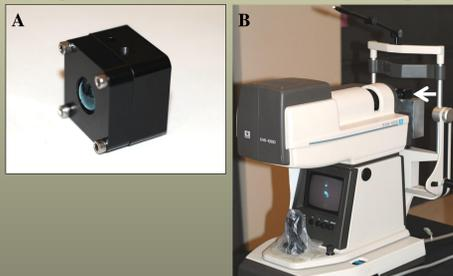
**Figure 1:** Light scattering measurements. A: Gross photograph of the customized dark eye model used to hold the IOL under immersion in BSS. The PMMA cornea is shown on the left; the model is filled with BSS though the holes shown on top. B: Photograph showing the Nidek EAS-1000 Scheimpflug camera. The eye model sits elevated on a metal bridge located on the chin rest (arrow).
